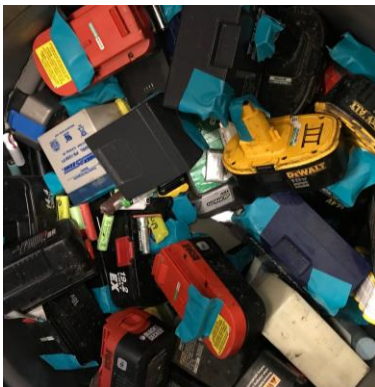
All different sorts of batteries. Taped with blue tape to ensure that they will not spark fires.
